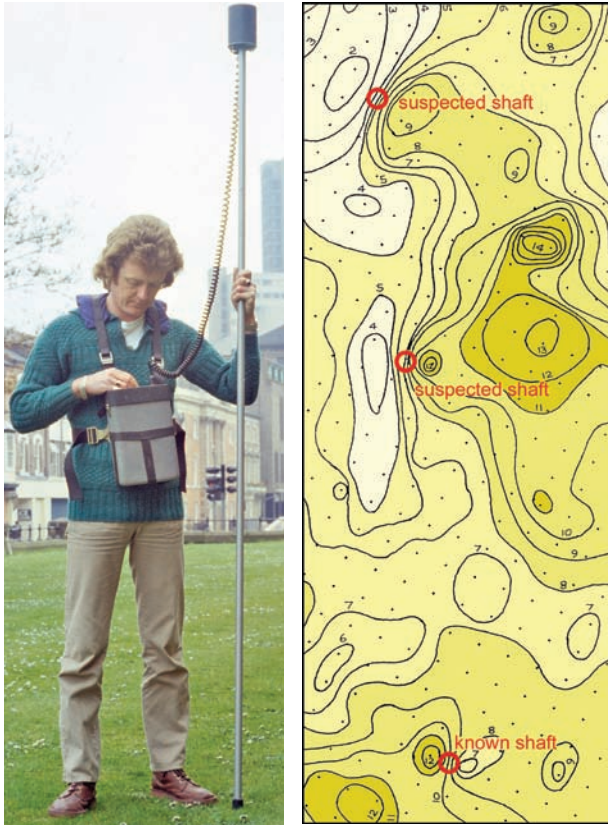
Proton magnetometer in use, and map of a magnetic survey on a site in the Derbyshire coalfield. Stations are on grid of 3 m; contours are at 100 nT intervals above base of 48,000 nT. Dipole anomalies lie over one known shaft and indicate the location of two more shafts.
