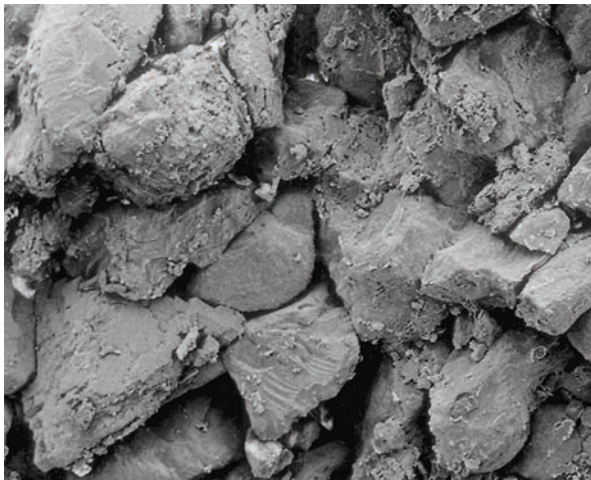
Electron microscope view of sandstone with quartz grains and weak flaky clay mineral cement. An original, partial, calcite cement has been removed by weathering.
