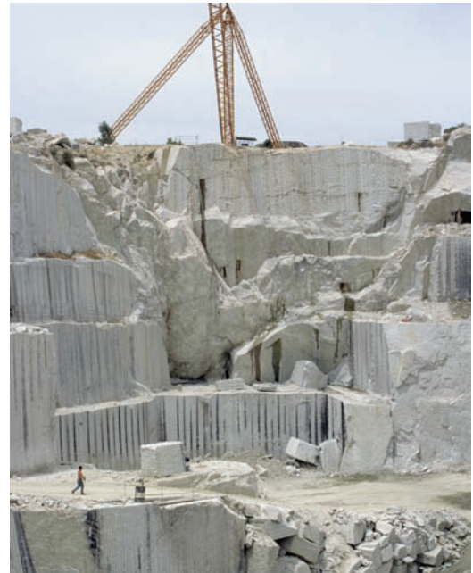
Granite quarry for dimension stone in Sardinia.
