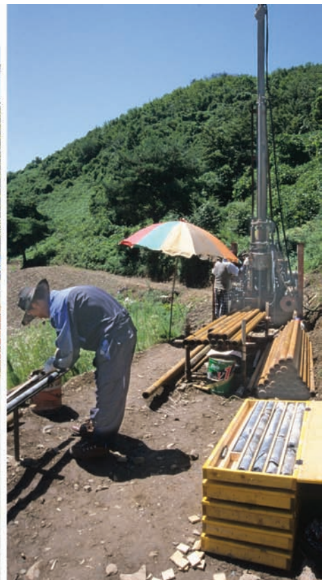
A diamond drill rig on a hillside in Korea, with core samples of strong limestone lifted from the split drill string and laid out in core boxes.
